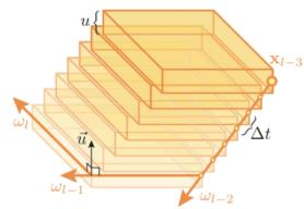
We replace distance sampling along  $t_{l-2}$  with deterministic "plane marching" (left) and select a uniform blurring kernel  $K_1(\mathbf{x}_l, \mathbf{y}_k) =$  $u^{-1}$  with blur direction  $\vec{u} =$  $(\omega_{l-1} \times \omega_l)/\|\omega_{l-1} \times \omega_l\|$  normal to the plane.
