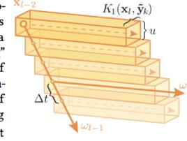
the ray offset of each beam to  $t_{l-1}^{(i)} = i\Delta t$ , where  $\Delta t$  is the step size. We select a blurring kernel which is uniform along one dimension,  $K_2(\mathbf{x}_l, \mathbf{y}_k) = u^{-1}K_1(\mathbf{x}_l, \mathbf{y}_k)$ , where *u* defines the uniform blur extent, and the direction of the uniform blurring is as in the figure above. The contribution of this estimator then becomes a sum,
